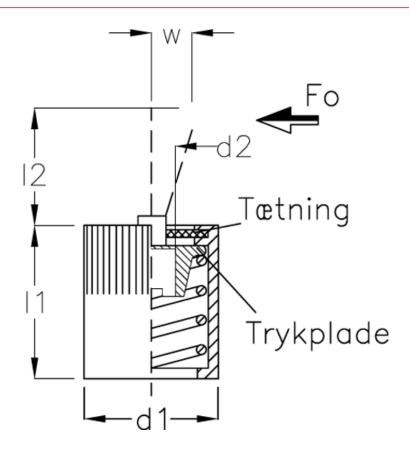
$\begin{array}{lll} d1 & = 10 \\ d2 & = M4 \\ d3 & = 10 \\ H & = 12 \\ I1 & = 12 \\ I2 & = 4.0 \\ screw driver & = GN 715.1-5 \\ Side power N at I2 = 50 \end{array}$
